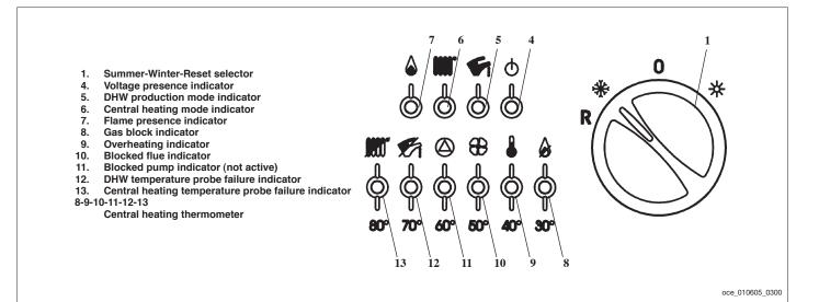
The lights 8÷13 display the temperature of the water in the central heating system (when not blinking).
