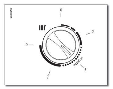
IMPORTANT: the range of heating flow temperature TM depends on the position of the jumper or switch T.RISC. ( see paragraph 13). The maximum possible temperature setting is 85 or 45 °C.
