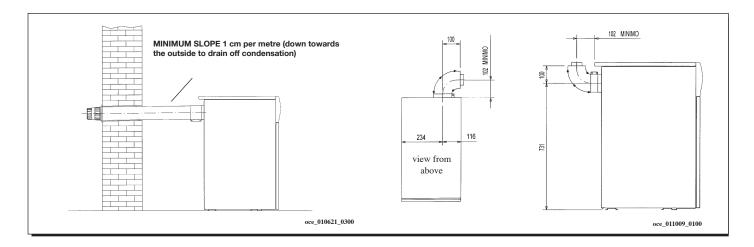
Adding a  $90^{\circ}$  bend shortens the total length by 1 metre. Adding a  $45^{\circ}$  bend shortens the total length by 0.5 metres.
