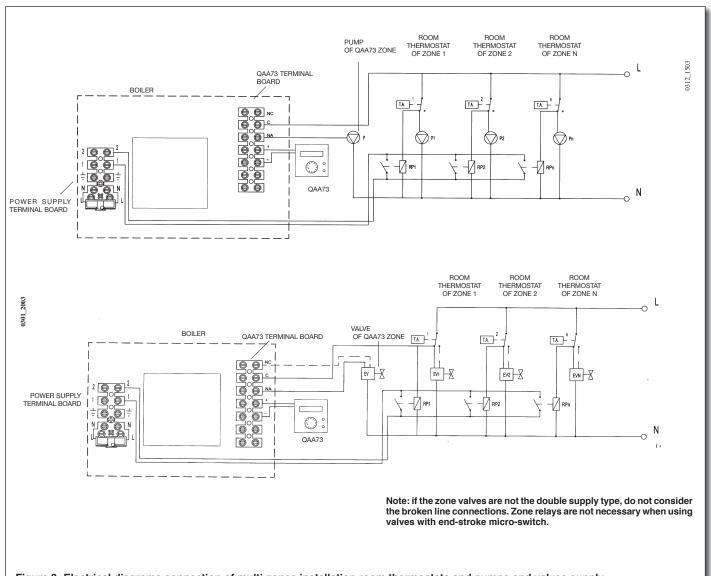
Figure 3: Electrical diagrams connection of multi-zones installation room thermostats and pumps and valves supply
