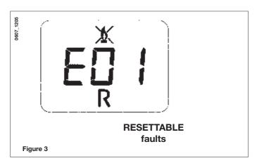
To RESET the boiler, press and hold down "R" for at least 2 seconds. If this fault persists, call the Authorised Service Centre.
